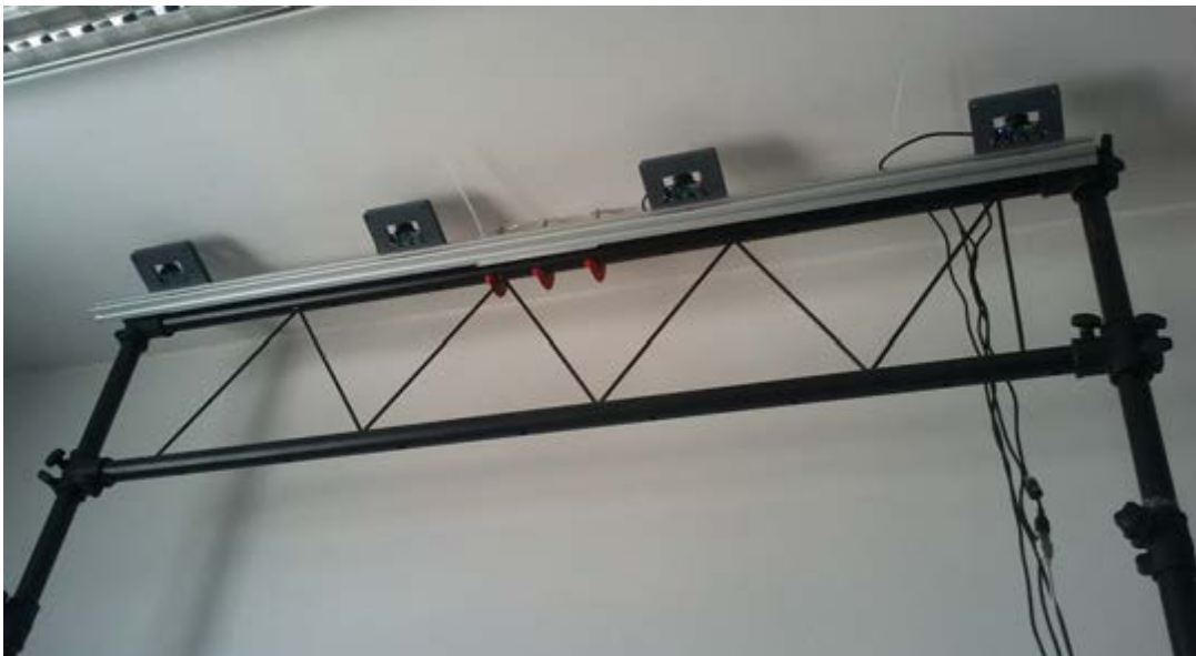
Figure 8.17: The simple camera network rig built for our setup.
