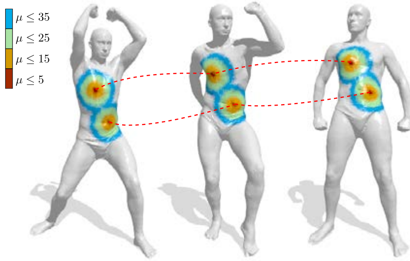
Figure 6.10: Effect of parameter \mu on the metric distortion term of Eq. (6.7). Increasing the value of \mu makes geometric validation more tolerant to distorted matches. In this real example on the SCAPE dataset, the colored regions show the admitted metric distortion for a pair of multi-way matches at different values of \mu . An optimal value for this parameter can be chosen such that a prescribed metric distortion is not exceeded (e.g., constrained to the orange area).
