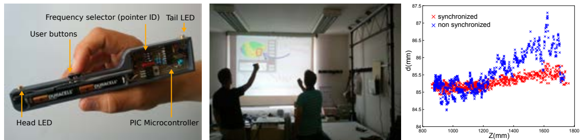
Figure 8.28: An interactive whiteboard system implements using the described design (left). Effect of the synchronization on repeatability (right)
