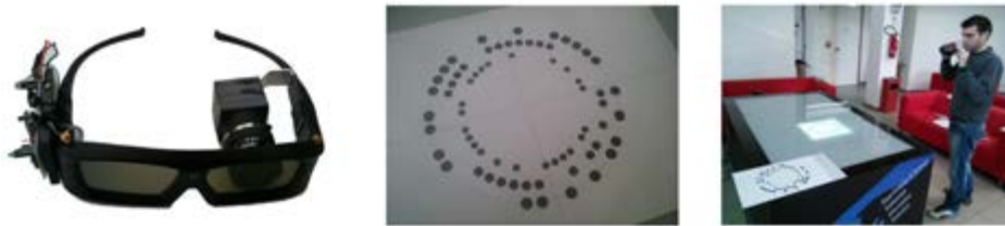
Figure 8.32: The modified glasses and the fiducial marker used for testing purposes.
