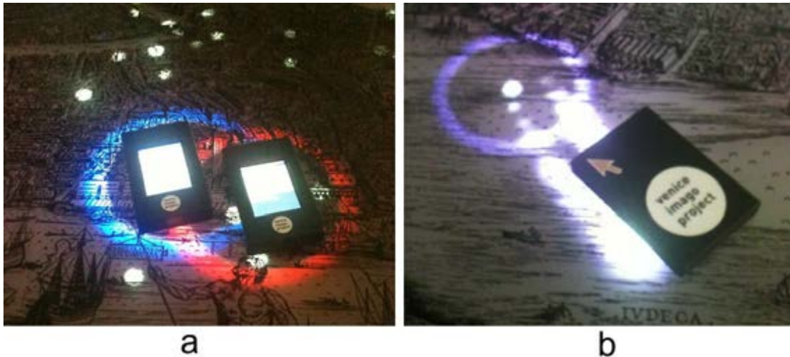
Figure 8.3: (a) The feedback on cursor location. (b) A visual suggestion to move.
