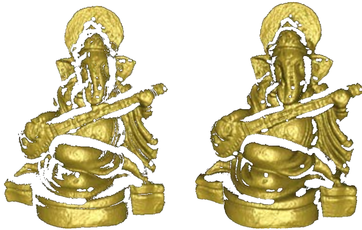
Figure 4.21: Reconstructed range-map triangulated with OpenCV calibration and rectification (Left) and our proposed method (Right).
