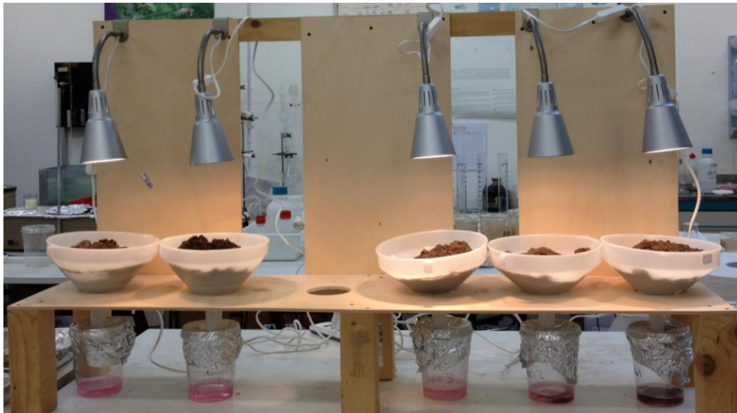
Fig. 12. The apparatus for the extraction of microarthropods in order to determine the QBS-ar index (Venice, Italy)
