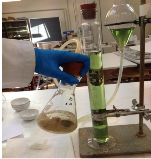
Fig. 9. Measuring total carbonate using calcimeter
