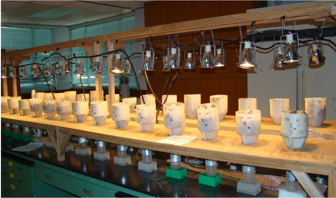
Fig. 13. The apparatus for the extraction of microarthropods for the determination of the QBS-ar index (IRRI, Manila)
