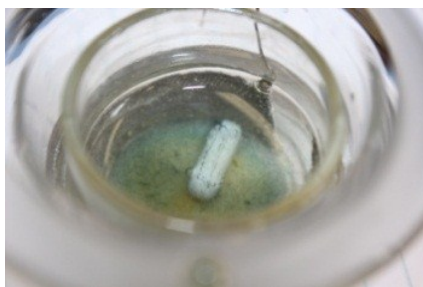
Figure 3.26 Yellow-green precipitate inside the CPE cell obtained by single-step CPE experiment on a aqueous solution of FeSO 4 (10 mM) and H 2 SO 4 (1 mM)
