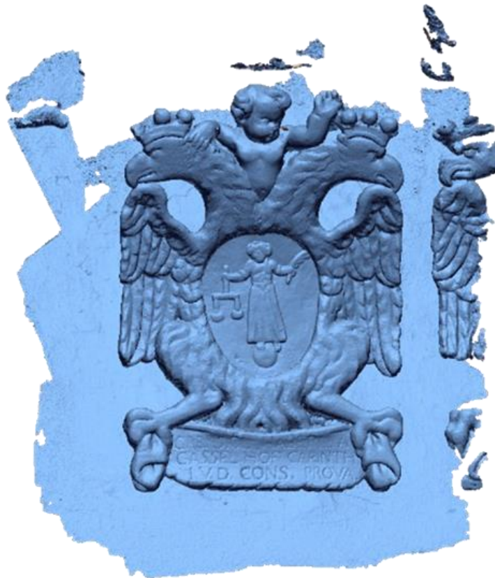
Figure 43 - Raw point cloud acquired with EinScan Pro HD
