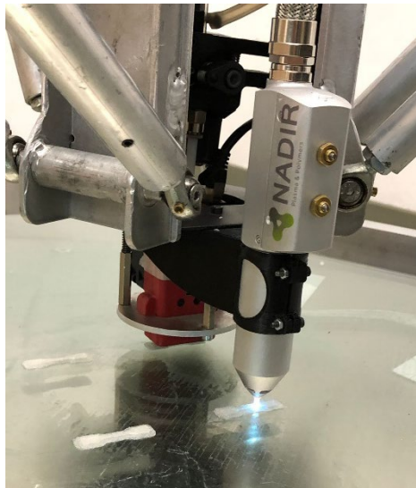
Figure 29. Plasma torch coupled with 3D printer. The torch has been provided by Nadir-tech, a company present at the scientific campus of Ca' Foscari University.
