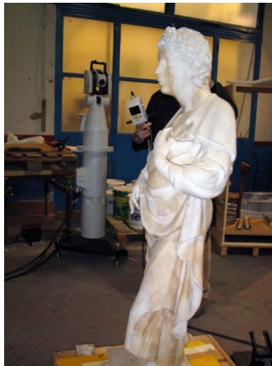
Figure 7. A three-dimensional replica of the Prophet's statue, made of polystyrene, thanks to the use of T-scan and Laser Tracker system [41].
